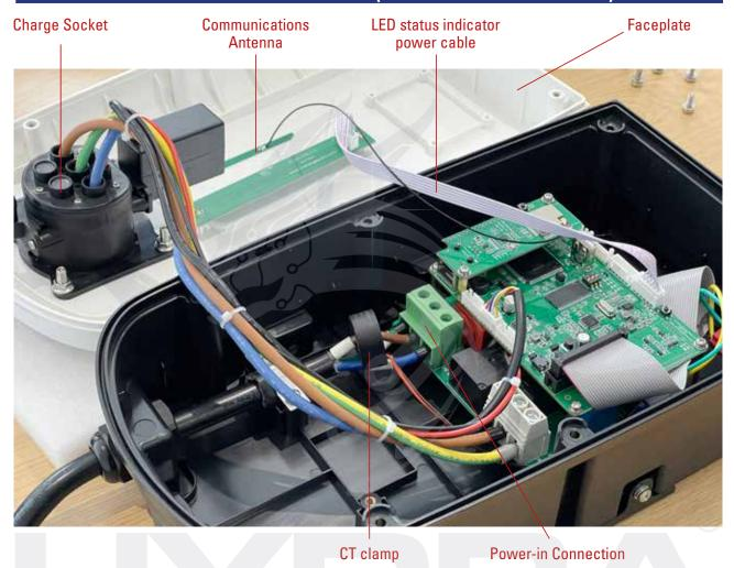
**Above** shows the single-phase 7kW Hydra Zodiac with the quick-connect tail attached. When disconnecting this to attach the power cable direct to the charger the CT clamp needs to be re-installed on the live feed.
