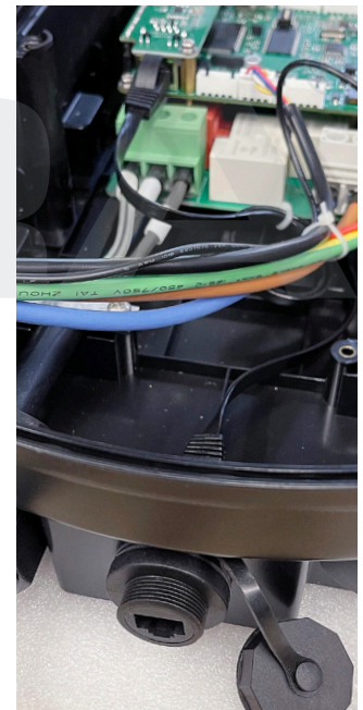
RJ45 Ethernet port (centre on some models)
